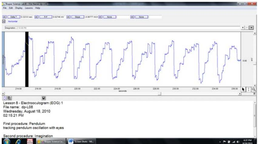
**Fig 8.15 Measuring the slope of a movement to determine that this example is not a saccade (slope =  $-0.06777\text{mV/s}$  which is less than  $-0.1$ ). The positive / negative value of a slope simply indicates direction right (+) or left (-) of the movement and should be ignored.**
