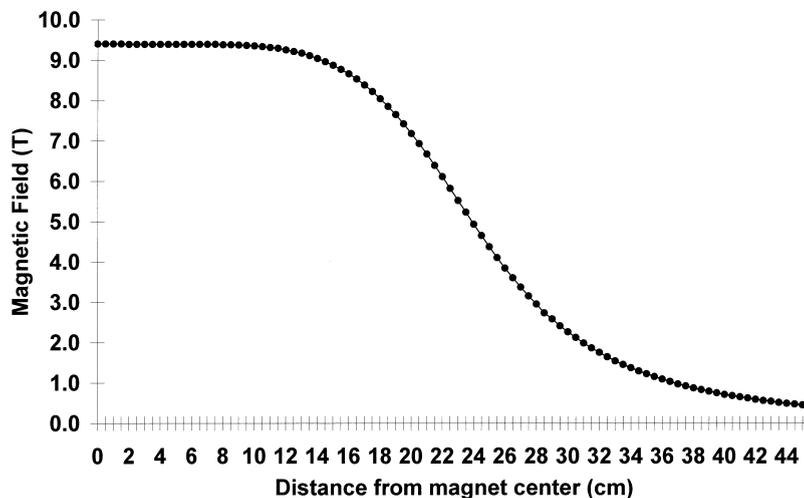
FIG. 1. Strength of the magnetic field measured in Teslas (T) from the center of the superconducting Oxford Instruments 400/89 magnet. 1 T = 10,000 Gauss. The 10-Gauss line is located 2.4 m from the center of the magnet.
